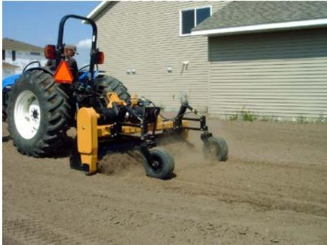
Use of a tractor power rake to properly condition topsoil and prepare ground for seeding. Removes all rock and debris from the soil, and promotes seed to soil contact.
